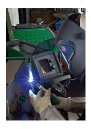
Development of new welding programs and processes, such as IAC for the Galaxy, causes the Special package to hold now almost 200 welding programs. Consequently, we have developed a program wizard, which is a quick method to finding the relevant welding program. On the display, under the easy-to-use program selection menu point, the user can choose wire type, wire dimension and shielding gas. Then the program is found in the memory and the user will be ready to weld, with no
